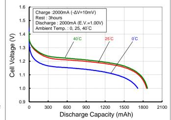
·Single cell performance and lifespan are greatly affected by usage and temperature conditions.
